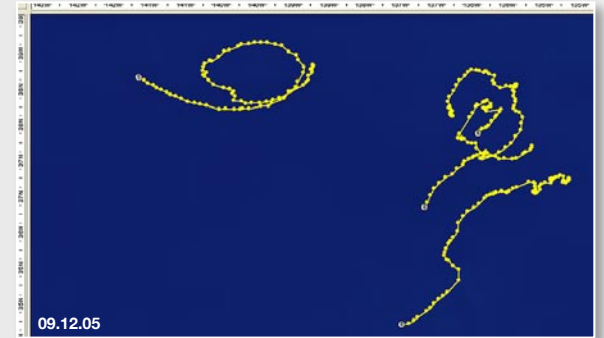
Four OTR-200 Buoys were attached to marine debris in the North Pacific Gyre. The graphic above illustrates the tracks of the buoys over a four-week time period. The top image shows the buoys' position relative to the North American West Coast. The yellow lines indicate each buoy's track. The points along the tracks represent days. Position information is provided in the upper and left borders.
